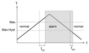
In the normal state the integrated LED is on, in the alarm state it is off, and this corresponds to its status when there is no supply voltage.
